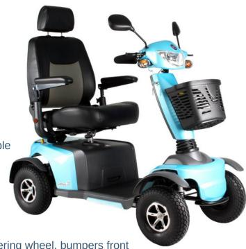
The Supernova has an angle adjustable steering wheel, bumpers front and rear, a headrest, impact resistant covers, a depth-adjustable seat slide and height adjustable and foldable armrests. The seat is rotated 360 °, the seat back is folded down and come back angle adjustment.
